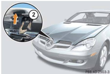
② Lever for opening the hood
